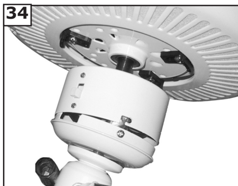
34 Attach switch cap to fan by lining up 2 slot ear holes and 1 screw hole and twisting cap. Then tighten the 3 screws.
