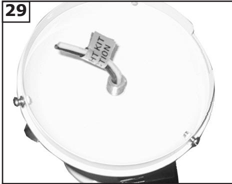
29 Remove switch cap housing from fan. Remove the plug of fitter. Install switch cap housing to light kit by turning clockwise to tighten.
