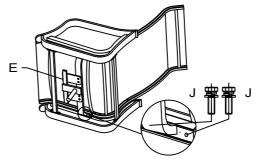
Connect chair seat support frame (E) with seat base (B). M8\*20 bolts (J) are used. Please tighten bolts to the end at this step.
