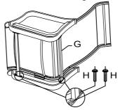
Connect chair seat support beams (G) with backrest (C and D). M6\*15 bolts (H) are used. Please do not tighten bolts to the end at this step.
