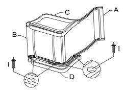
Connect chair back (A) with seat base (B) and armrests (C and D). M6\*30 bolts (I) are used. Please do not tighten bolts to the end at this step.
