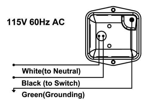
**Figure 2**: Wiring Diagram - Single speed. 115-volt connection. for ILG8SF18S, ILG8SF30S, ILG8SF36S
