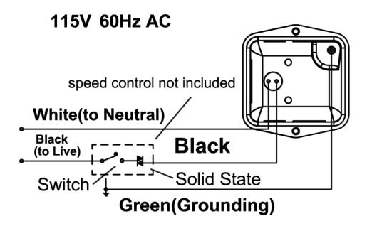
Figure 1: Wiring Diagram - Speed Controllable. 115-volt connection.
