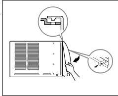
10. Lift the inlet grille and secure it with a Type A screw through the front grille.
