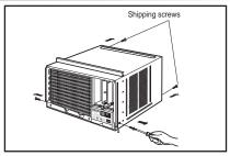
2. Slide the unit from the cabinet by gripping the base pan handle and pulling forward while bracing the cabinet.
