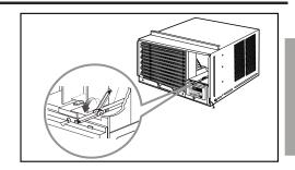
9. Attach the front grille to the cabinet by inserting the tabs the grille into the slots on the front the cabinet. Push the grille in until it snaps into place.
