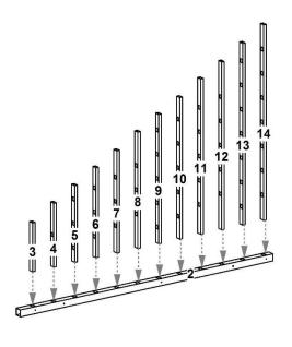
Lay out one right post (part 2). Starting at bottom (end with hole 4" from post end), insert cross rails from shortest to longest (part 3-14)
