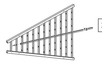
Starting with center hole, insert 84" vertical rail (part 15) through cross rails.
