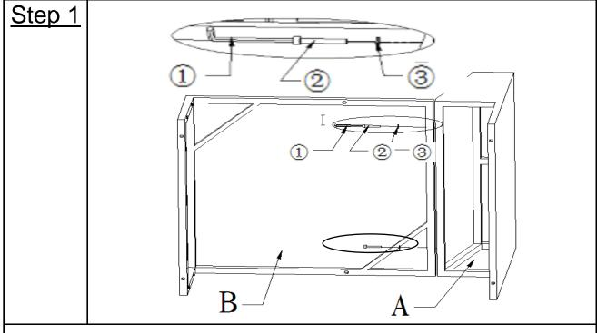
Open the carton and place all the parts onto a clean, non-marring surface. Attach Chair Back(A) to Chair Seat(B) using Bolt(2) and Washer(3) with Allen Key(1) as shown above.
