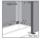
On walls where tile will reach the floor, determine whether floor is level by measuring distance to desired tile height on both sides of area to be tiled. If there is a difference (e.g., the floor is lower on one side), lay one vertical row of tile from highest point down to floor. Affix tiles with dabs of mastic.
