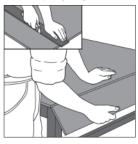
– Power saw: Use a low-RPM portable saw with 3-1/2" carbide-tipped blade. To make cutouts for pipes and fixtures, use utility knife to cut through mesh on both sides of panel and punch out with a hammer from back side. Or, use an electric drill with a hole-saw bit.
