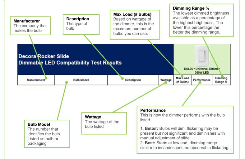
If a rating for a particular bulb/dimmer combination is not provided, it could indicate inconsistent results or test results not available at this time. As additional test results for current and newer bulbs and dimmers are obtained, the compatibility chart will be updated.
