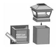
To attach your post cap to the post, apply PVC glue to the underside of the post cap before placing the cap firmly on the post.
