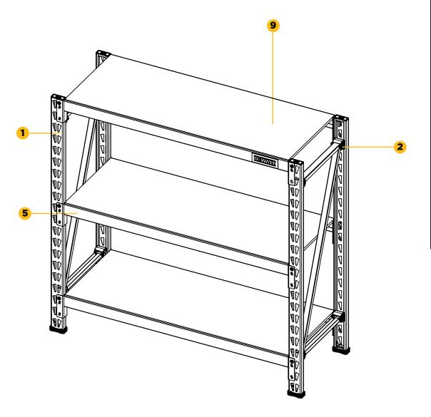
*Tools Required for Rack Assembly:* 4 mm Hex Key (included) OR 4 mm Hex Bit (included); Rubber Mallet (not included)
