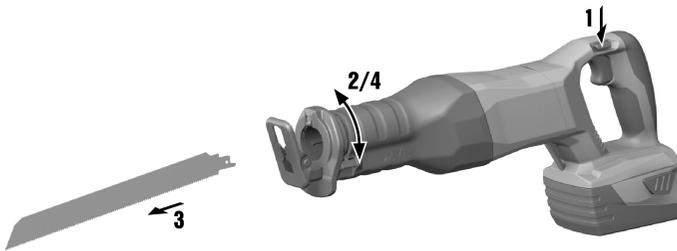
1. Activate the transport lock or separate the battery from the power tool.
