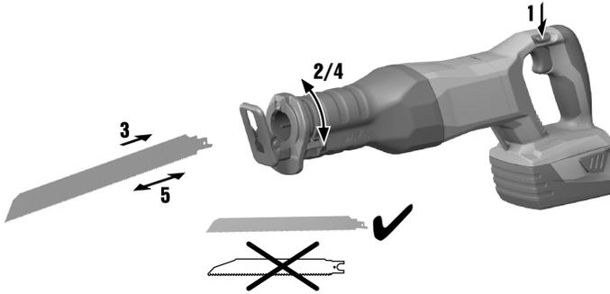
1. Activate the transport lock or separate the battery from the power tool.
