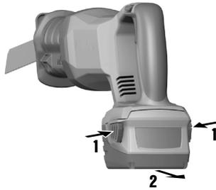
1. Press the two release buttons and hold them in the pressed position.
