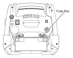
Step 3: Remove the fuse cover and replace the fuse.
