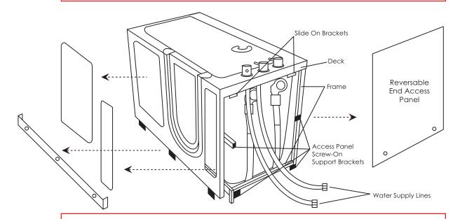
**WARNING:** Lift and carry the tub only by the frame. Protect the bottom of the tub to avoid breaking the air jets positioned on the bottom of the tub.
