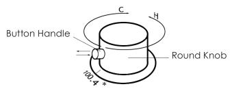
\*The button knob stops here at 100.4 Fahrenheit. To adjust to a hotter temperature past 100.4 F, press the button knob in while turning the handle counter clockwise
