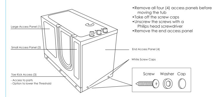
**WARNING:** Do not carry the walk in tub by the panels. Be careful when carrying the tub, avoid front panel contact with the floor or stairs to prevent damages. Make sure no loose parts are hanging down. Remove all four (4)access panels before carrying the tub to prevent them from falling out and breaking.
