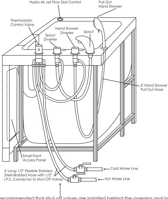
**NOTE:** It is recommended that shut off valves are installed behind the opening and in reach from the small access panel.
