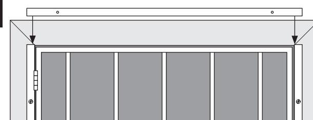
Position the top header jamb (**C**) across the top of the two side jambs. Make certain there is a minimum 1/8" space between the header and the top of the door frame, and that the header is level.
