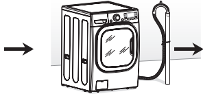
Connecting the drain line
