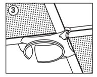
3. With the ceiling grid slotted between the Stingray's fins, push until Stingray locks into corner. You are now ready to run your wire.
