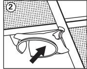
2. Slide Stingray into the corner of the ceiling grid, positioning the upper fins above the grid, and the lower fins below the grid.
