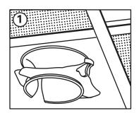
1. Remove both tiles in the corner of the ceiling you wish to install the Stingray, and position the Stingray tail down as shown.
