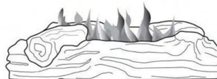
Figure 20 - Correct Burner Flame Pattern Showing Blue Flame with Yellow/White Tips
