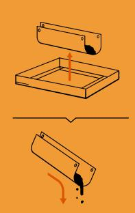
Remove the ashes from your pit. This can be done by dumping the pit, by using a shovel, or by removing the Fire Mesh. To remove the Fire Mesh look for the two bottom Ember Guards from Step 2 of the assembly. Simply place hands in the middle of each Ember Guard and pull straight up keeping the Ember Guards parallel to the ground. This should remove all four Ember Guards as well as the Fire Mesh in one unit. The Fire Mesh can then be funneled, and the ash dumped out from it
