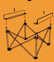
Pay close attention to which Ember Guard has the badge, this should be set aside until Step 3. Two Ember Guards should be placed on the frame parallel from one another. Guide the upright pole of the frame through the pre-cut holes in the Ember Guards.
