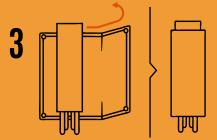
Place the Fire Mesh with the folded side up on the ground. Place the frame and Ember Guard construction on top of the Fire Mesh and roll together tightly. Repeat for Heat shield if applicable.
