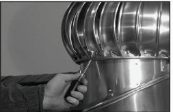
10.After installing check to see that whirlybird turns freely. In transportation it may have shifted slightly. If necessary, minor adjustment may be made by gently prying lowest point of turbine upward to remove any wobble.
