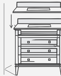
② Install Counter Top.
