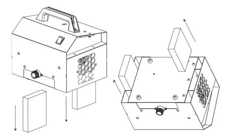
Check the condition of filter carefully and replace if necessary.
