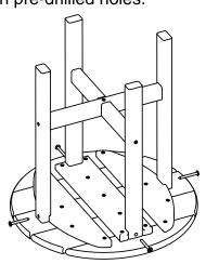
Step 3 Connect the braces using (1) 8x11/4 Screw.
