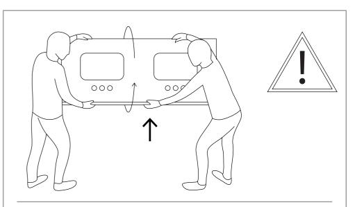
While turning around the double sink counter tops, always add support from the centre for safety
