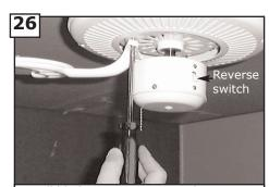
Install blades to motor using the 10 motor screws provided. Tighten screws securely. Setting the reverse switch in the down position will result in downward airflow and setting the switch in the up position will result in upward airflow.
