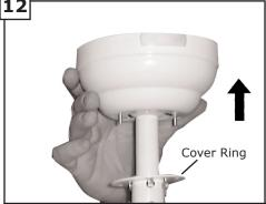
Lift Conopy allowing the 2 studs to protrude through the canopy.
