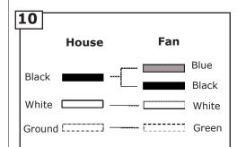
Connect black and blue wire from fan to Black or (Hot) wire from house. Connect White wire from Fan to White (Neutral) wire from house. Connect Ground leads from mounting bracket and downrod to Ground lead from house. Refer to Safety Tips section of manual.
