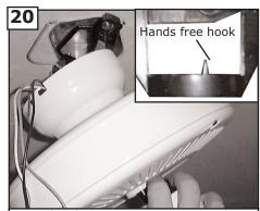
Hang fan from mounting bracket by the hands free hook into a closed hole on the edge of the Canopy.
