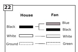
Connect black and blue wire from fan to Black or (Hot) wire from house. Connect White wire from Fan to White (Neutral) wire from house. Connect Ground leads from mounting bracket and downrod to Ground lead from house. Refer to Safety Tips section of manual.
