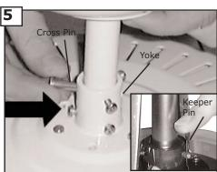
Insert downrod into yoke on top of the Fan Body. Align the hole in the Downrod with the hole in the Yoke. Insert the Pin through the Yoke and Downrod until the point appears on the other side. Install the Keeper Pin
