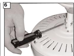
Tighten the 2 Set screws on the Yoke once the downrod is in place. Check motor for shipping stabilizers and remove if present.
