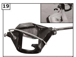
Install 2 of the screws to the side panel corresponding to the open slotted holes on the canopy upper rim. Remove the all thread studs from the lower part of the mounting bracket.
