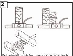
Before installing this fan make sure the outlet box is properly installed to the house structure. To reduce the risk of fire, electric shock, or personal injury, mount to outlet box or supporting system acceptable for fan support. (Mounting must support at least 35
