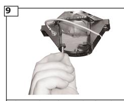
Make sure the studs protruding from the bottom of the Mounting bracket are in-stalled with threads all the way through
