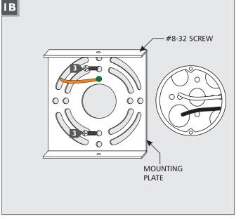
3 Attach the mounting plate to the electrical box using the two #8-32 screws provided.
