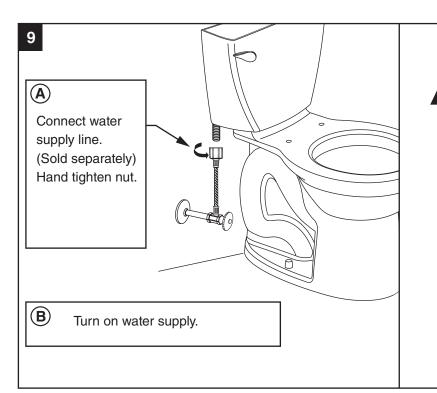
**WARNING:** Overtightening of water supply line nuts could result in breakage and potential flooding. If the connection leaks after hand tightening, replace the supply line. Do not use any type of sealant on the water supply connection. Use of plumber's putty, pipe dope, or any other type of sealant will void the warranty.
