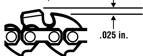
RAKER (DEPTH GAUGE) CLEARANCE
