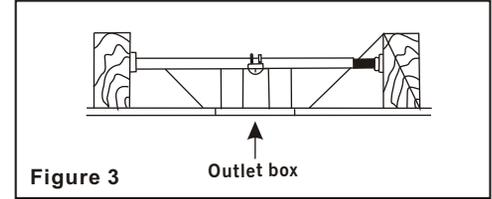
To hang your fan where there is an existing fixture but no ceiling joist, you may need an installation hanger bar as shown in Figure 3 (available at any Home Depot store).
