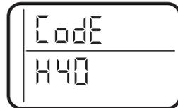
7. To change the code number, press the ▲ UP or ▼ DOWN button until the correct code shows.
