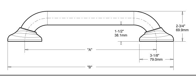
MATERIALS: Grab bar is constructed using 1-1/4" diameter 20 gauge 304
