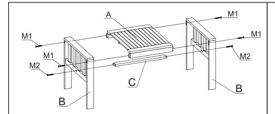
Step 1: attach table leg frame (B) to table top (A) & low cross bar (C), using screws (M1 & M2). Fully tighten using Allen Key (M7)
