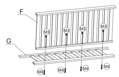
Step 1: Fix the seat bench (F) to Backrest (G) using Bolts (M4) & Nuts (M3). Fully tighten using Allen Key (M7)
