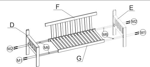
Step 2: insert Wooden dowel (M6) into the hole in bench seat (G) then attach the right leg frame (D) to the assembled frame. Tighten using Allen Key (M7). Repeat for the left leg frame (E).Do not fully tighten Screw until all are installed.
