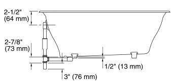
No change in measurements if connected with drain illustrated.
