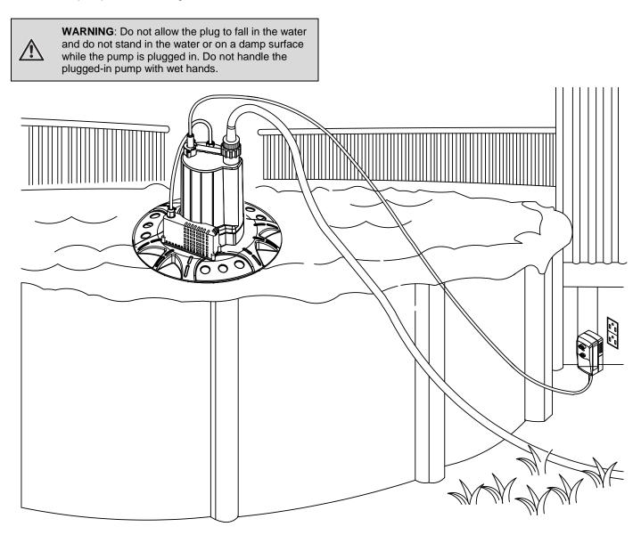
**NOTE**: The float switch is located in the cage on the side of the pump. Keep this cage clean so the float switch can operate properly.
