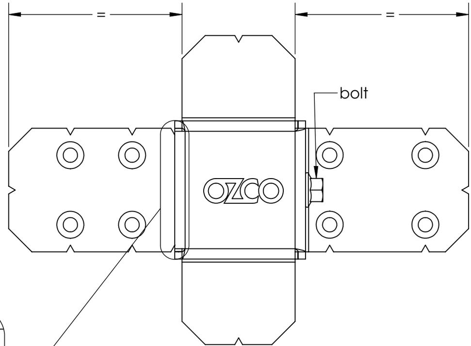
line up edge and alignment feature by turning bolt to evenly center assembly prior to installation
