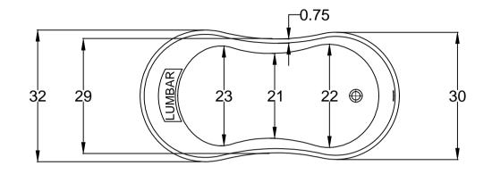
OVERFLOW IS INTEGRAL TO THE TUB
