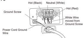
1 Remove 5-inch (12.7 cm) of the outer covering from the wire. Remove 5-inch of insulation from the ground wire. Cut off approximately 1.5-inch (3.8 cm) from the other three wires and strip 1 inch (2.5 cm) insulation from each wire. Bend the ends of the three shorter wires into a hook shape.
