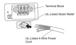
**5** Transfer the dryer's ground wire from behind the green ground screw to the center screw of the terminal block.
