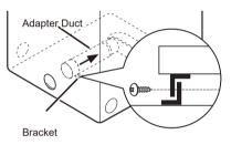
3 Insert the 4-inch (10.2 cm) elbow through the rear opening and press it onto the adapter duct. Be sure that the male end of the elbow faces down through the hole in the bottom of the dryer. Secure it in place with duct tape. Attach the cover plate to the back of the dryer with the included screw.
