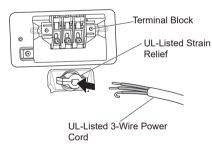
5 Attach the two hot leads (black and red) of the power cord to the outer terminal block screws.
