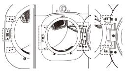
3 Remove the four decorative screws on the left using a screwdriver.
