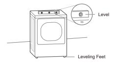
• All four leveling feet must rest solidly on the floor. Gently push on the top corners of the dryer to make sure that the dryer does not rock from corner to corner.
