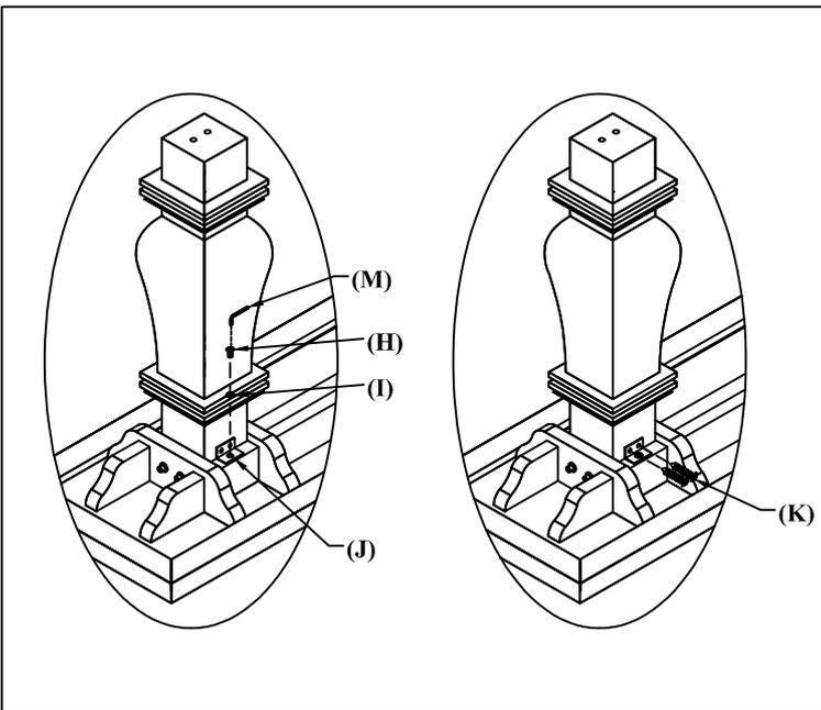
Step- 03 Use allen key (M) to tighten the metal angle (J) with pen head allen bolt (H) and washer (I). Do not fully tighten. Use a screw driver to tighten metal angle (J) to the leg (B) with wooden screw (K). Once completed, tighten allen bolt (H) fully.
