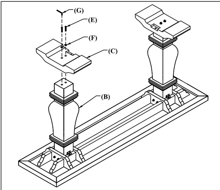
Step -05 Place the base (C) on the leg (B) and secure with allen bolt (E) and washer (F) with allen key (G).
