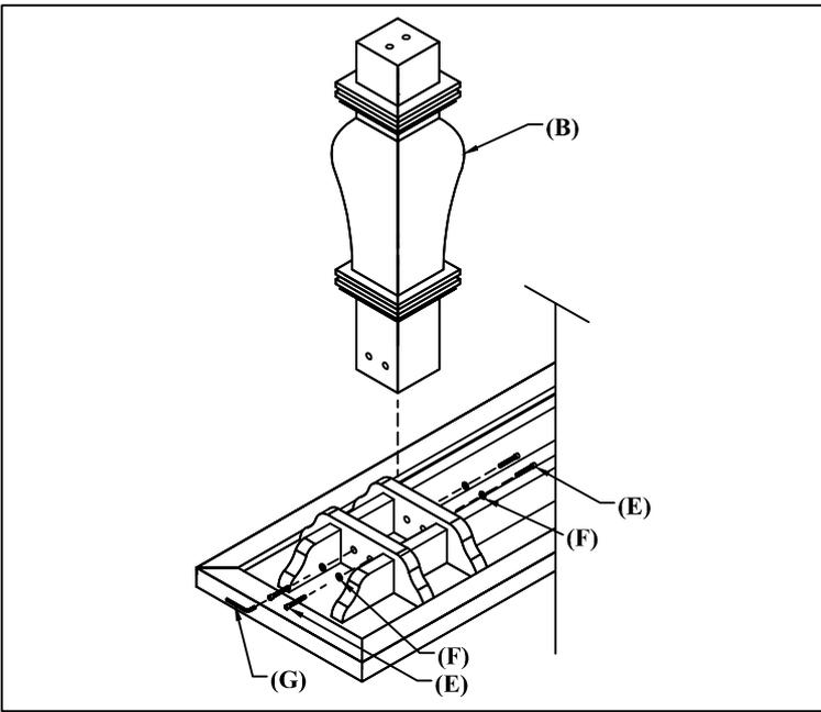
Step -02 Align the holes in the leg (B) and frame of top (A). Using the allen key (G), tighten the washers (F) and allen bolts (E).
