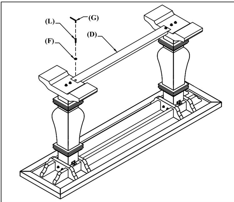
Step -06 Affix the bottom support (D) to leg bases by tightening allen bolts (L) and washers (F) with allen key (G).
