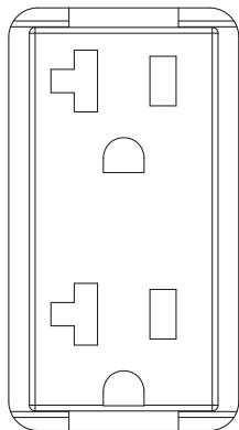
**Figure 7 - 120/240 VAC, 30 Amp Receptacle**
