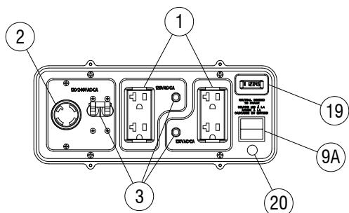
**Figure 3 - Generator Controls**
