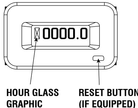
When the hour meter is in the Flash Alert mode, the maintenance message will always alternate with elapsed time in hours and tenths. The hours will flash four times, then alternate with the maintenance message four times until the meter resets itself.
