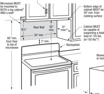
Locate 120V/60Hz grounded outlet inside upper cabinet
