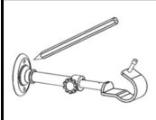
1. Using the bracket as a template, place it in the desired location. Mark holes.
