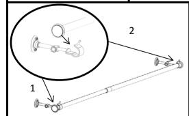
9. Place the rod into the brackets (1)(2) (Curtain not shown) For additional support, install the extra bracket(s), if needed (141-274 cm & 274-427 cm only).
