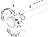
8. Remove End Cap by turning counterclockwise (1). Place the curtain onto the Cap by screwing threaded end into hole in clockwise motion until seated. (3)
