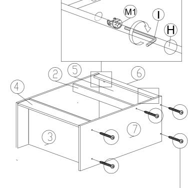
Fix Panel (2,3,4,5,6) onto panel (7) by inserting dowels (A) onto non-thru at panel (7) use allen key (1) to tighten screws (G) from the thru-holes of panel (7) and after that insert minifix cap (H).
