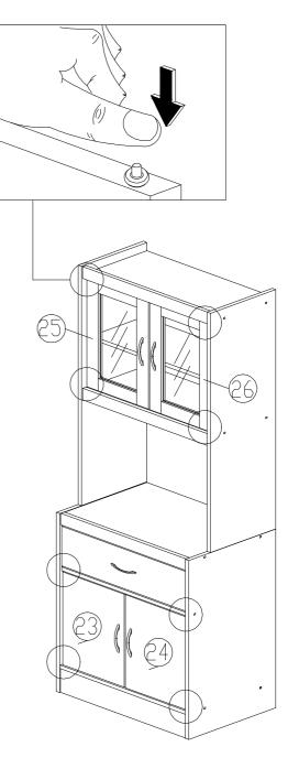
Fix down door panel (23,24) by pushing and slotting the door support (K) onto each holes at bottom of panel (3) and top panel (2).
