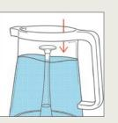
Remove the Carafe Lid and fill the Carafe with cool or room temperature water. Ensure that the spout on the Carafe Lid is closed for the brewing. The '\_\_\_\_' symbol should align with spout. This represents that it is closed.
