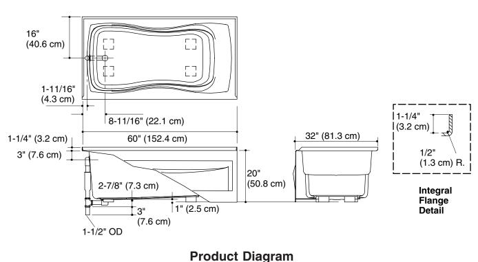
No change in measurements if connected with drain illustrated.
