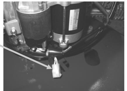
Attach the positive (red) and ground (black) battery terminal wires to the battery to provide power to the electric starter.
