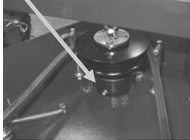
**Note:** The lower spindle bearing is sealed on the bottom and open on the top. The upper spindle bearing is sealed on both sides. Failure to frequently replenish grease will cause premature lower bearing failure. Frequent application of grease to this bearing is critical to achieving long spindle life in harsh duty environments.
