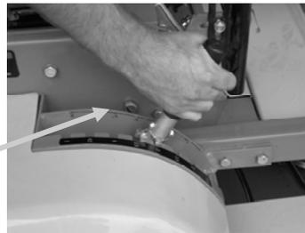
**Note:** After mowing, remember to pull the deck to its highest position to avoid scraping and any other kind of damage to the blades or deck.
