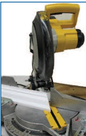
**Step 2** - Put the mating piece of trim on the saw in the **right hand compound position**. Then move the table angle gage to the opposite calculated angle, and cut. The miter joint is ready to be put together.
