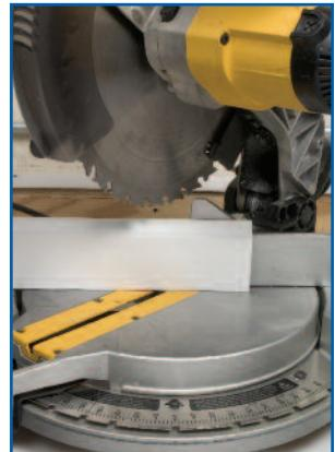
**Step 1** - To accomplish this, place the trim on the saw table in the **left hand vertical position** and rotate the angle gage "clock wise" to 45°, or the desired angle setting, and make the cut.
