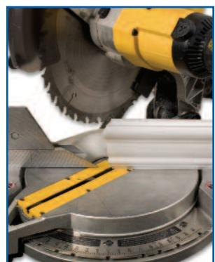
**Step 1** - To complete this, place the trim on the saw table in the **right hand vertical position** and rotate the angle gage "clock wise" to 45°, or preferred angle setting, and make the cut.
