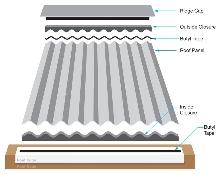
Start at the eave by positioning a line of butyl tape on the roof edge. Remove the release paper on the tape and gently embed the foam closure strip.
