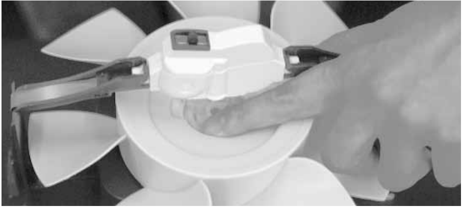
Fig 4. ... Push the coupling down ...
