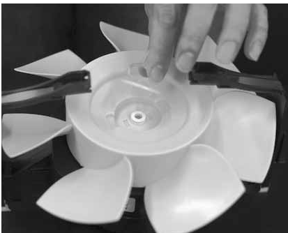
A.... Place the rubber coupling into the locking ring ...
