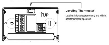
Mount your new thermostat base using the supplied screws. Drill holes and insert wall anchors to secure the thermostat base to the wall, if necessary.
