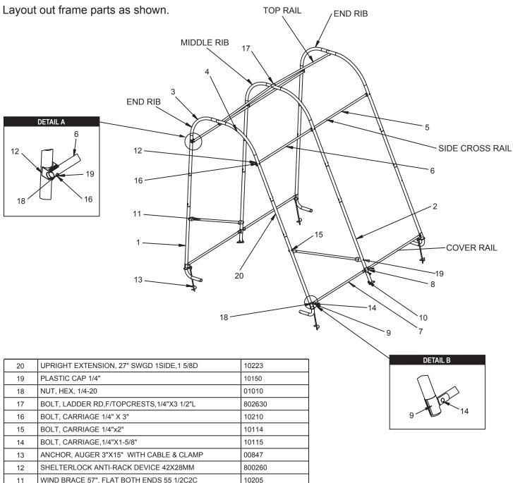
WIND BRACE 57", FLAT BOTH ENDS 55 1/2C2C 10 FOOT PLATES 1-3/8" DIA 10270 9 3-WAY COVER RAIL CLAMP 1 5/8" PIPE 10112 8 4-WAY COVER RAIL CLAMP 10111 CROSS RAIL PLAIN ENDS 45 3/4"L, 2 HOLES 10110 7 6 CROSS RAIL 48-1/2"X1.163",PLAIN ENDS 2 H 02031 5 CROSS RAIL 50-1/2"X1.163", 1 SWDG 2 HOLE 02030 4 SIDE BEND PLAIN 74"X1-5/8"DIA 800469 SIDE BEND SWDG ONE SIDE, 74"X1-5/8" DIA. 3 800468 2 UPRIGHT 56"X1-5/8" DIA. 10273 UPRIGHT W/LEG SWGD ONE SIDE, 63"X1-5/8" 1 ITEM DESCRIPTION PART NO. NO
