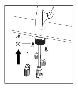
Adjust direction of faucet body (2) so that handle is on right side of faucet. Tighten mounting nut (5B) until snug. Tighten mounting screws (5C) to nut with Phillips screwdriver until snug
