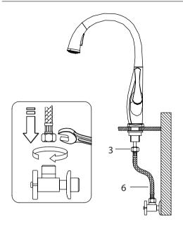
Connect waterlines (6) to hot and cold copper lines (3). Connect waterlines (6) to angle stops. Tighten both ends of waterlines with a wrench until snug. Turn on hot and cold angle stops and check for leaks
