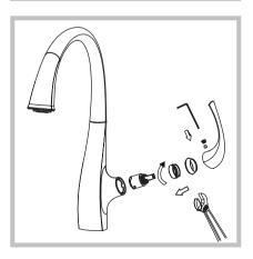
**Step 3:** Place the new cartridge in the handle seat. Secure the cartridge with the locking nut and assemble the handle
