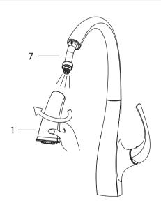
Remove spray head (1) from spray hose (7). Hold tip of spray hose (7). Turn faucet on and let the water run for 60 seconds to flush any debris
