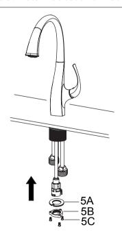
Insert faucet body (2) into hole in countertop or deck plate assembly . Install mounting hardware (5A, B & C) from underneath the countertop
