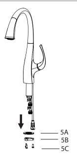
Remove the mounting screws (5C), mounting nut (5B), and rubber & metal washer (5A) from the mounting pipe
